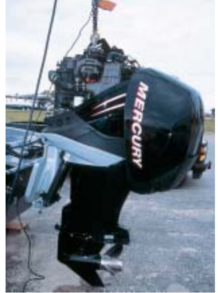
■ The engines were weighed with cowlings, props, steering cylinders and hoses attached.
