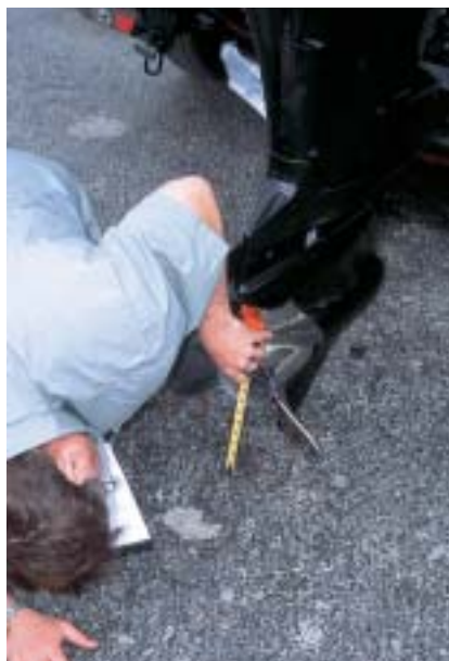
■ Propshaft height as tested varied from 5 1/4 inches below the pad (Verado) to 6 inches below the pad (Yamaha), with the OptiMax and Suzuki coming in at 5 1/2 and 5 3/4 inches, respectively.
